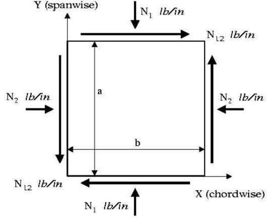
Figure 2: Typical wing cover panel
