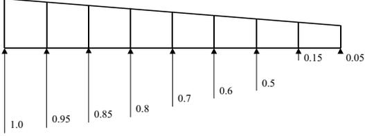
Figure 5: Normalized span-wise pressure distribution
