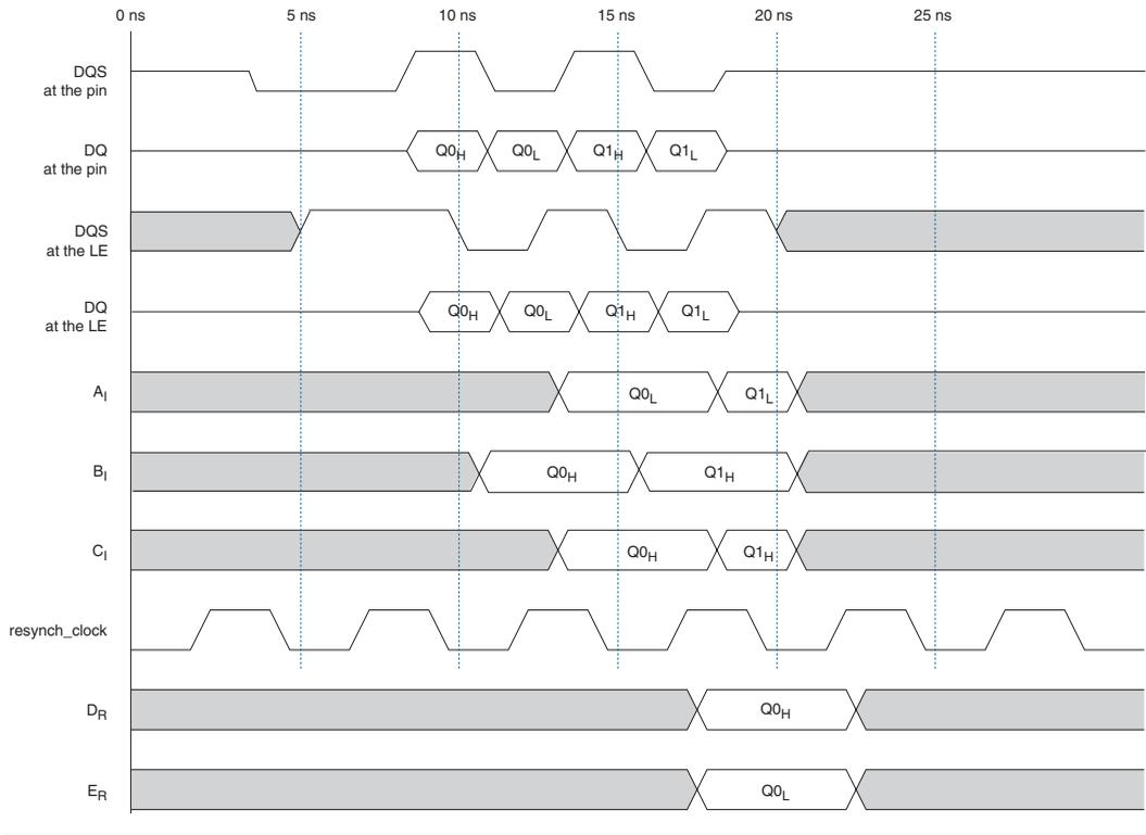
The first falling edge of the DQS signal at the LE register occurs at 10 ns. At this point, data Q0<sub>H</sub> is clocked in by register B<sub>I</sub> (waveform B<sub>I</sub>). At 12.5 ns, data Q0<sub>L</sub> is clocked in by the active high register A<sub>I</sub> (waveform A<sub>I</sub>) and data Q0<sub>H</sub> passes through the register C<sub>I</sub> (waveform C<sub>I</sub>). In this example, the positive edge of the resynch\_clock signal occurs at 16.5
